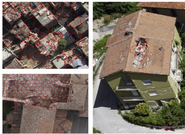
Figure 4: Super-pixels of UAV images, that were voted as damages based on the classified CNN features by the Support Vector Machine (SVM) classifier, are highlighted as red polygons in the subset of UAV images of Kathmandu (left-top), Mirabello (left-bottom) and L'Aquila (right) [18]
