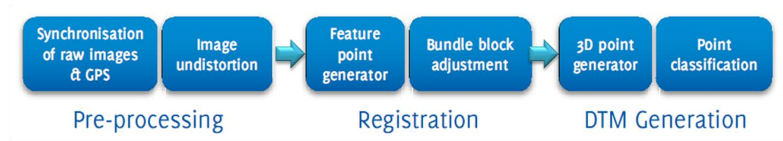
Figure 4: Image processing and output generation stages.
