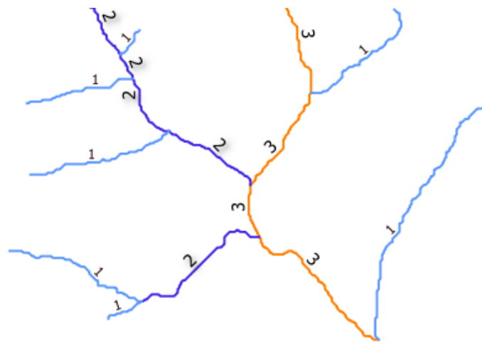
Figure 9: Delineated stream segments. At every confluence, a new segment is created. The numbers indicate the order of the stream according to Strahler rules.
