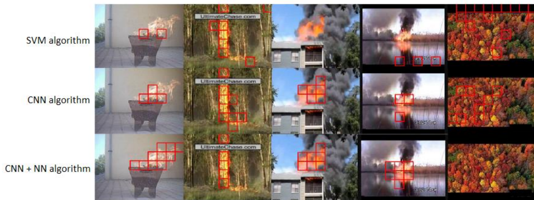
Figure 6: Detections results of different classifiers, from top to bottom, SVM algorithm, CNN algorithm, and CNN and NN algorithms [23]
