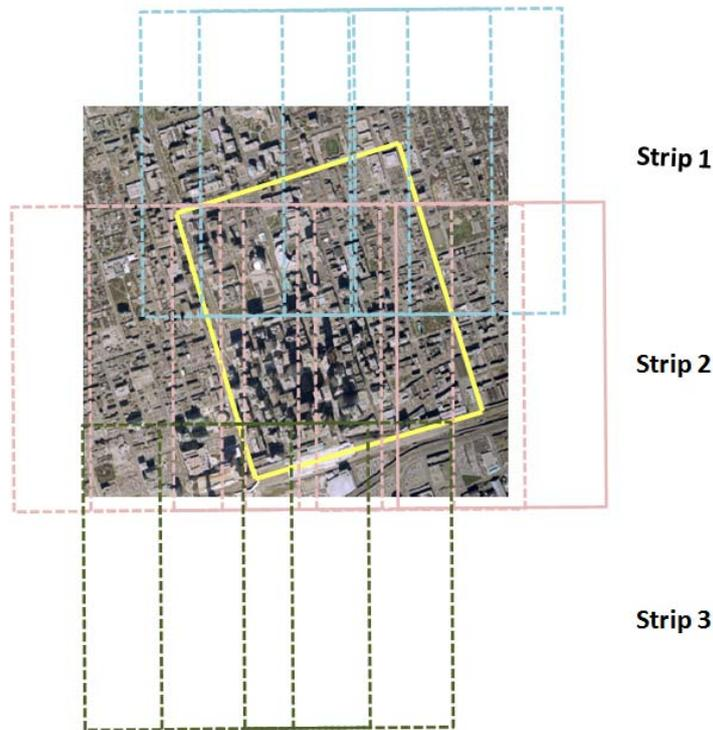
Figure 9: Image configuration for the downtown Toronto test site.
